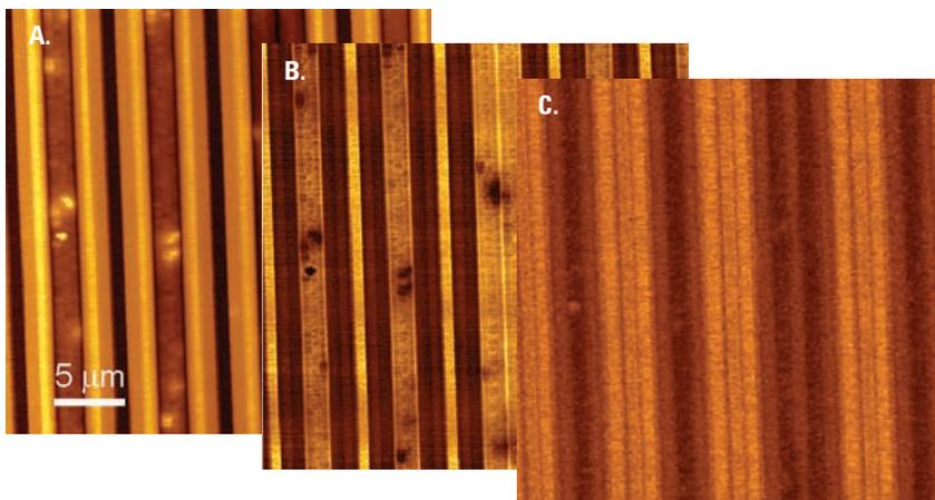
Figure 5. Simultaneous topography (A), capacitance (B), and dC/dV (C) images of SiGe transistor device. Both capacitance and dC/dV images resolved the underneath dopant structures not seen in the topography. Images obtained with 5420 in Scanning Microwave Microscopy (SMM) mode.
