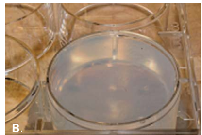
Figure 4. A. Concentric-cylinder sample holder. B. Agarose gel as supplied in a well plate.
