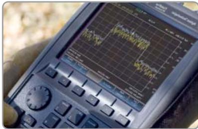
In order to facilitate LTE technology trials and its deployment, Agilent Technologies has developed an LTE receiver drive test system for air interface troubleshooting and optimization, and a handheld RF analyzer for cell site test and interference hunting to help you tackle the challenges of LTE deployment.
