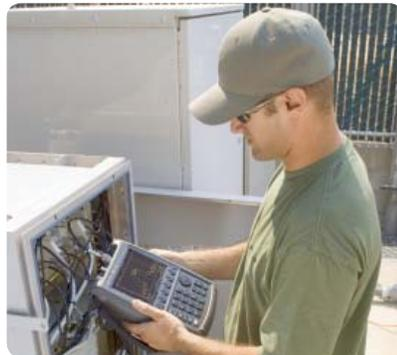
Figure 6. Cable and antenna analyzer
