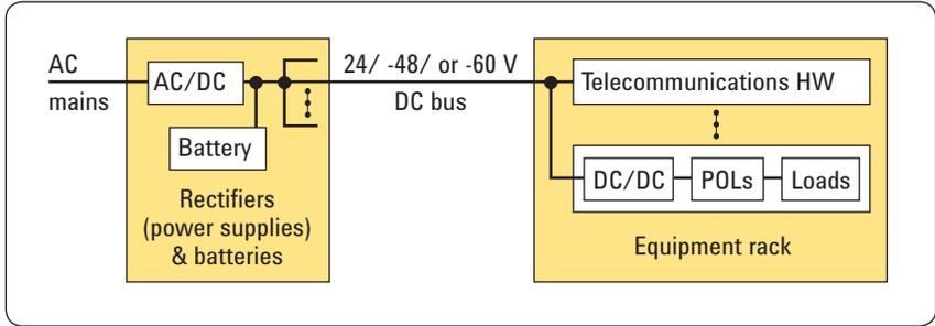
Figure 1. Telecommunications low voltage DC power distribution
