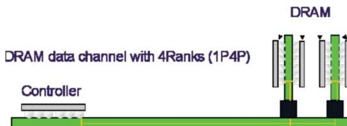
Figure 6. Multidrop memory bus example
