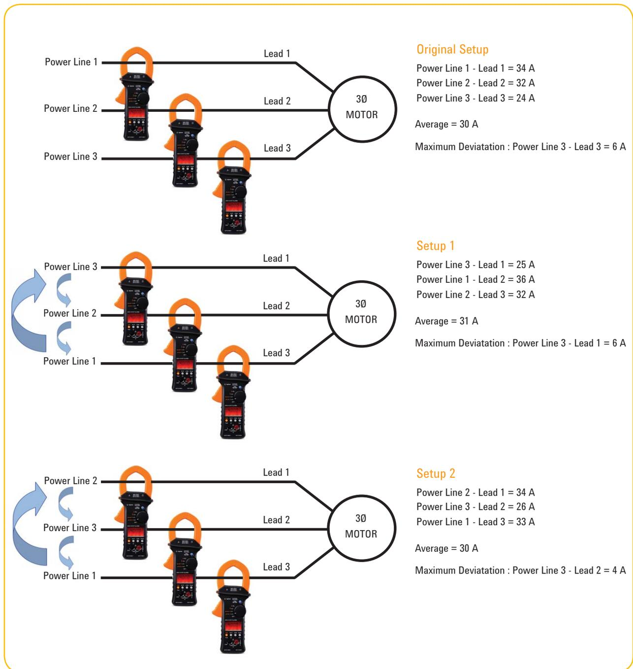
**Figure 1.** Steps to identify the source of unbalance
