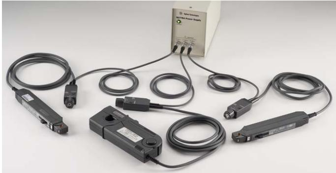
Figure 1. With a current probe, characterizing the current profile of a DUT is as simple as clamping the probe around a conductor.
