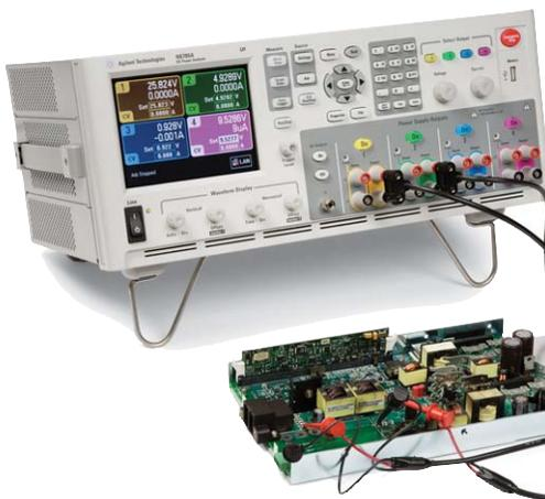
The N6705A has a current measurement bandwidth of 10 kHz. This can be a limitation when characterizing dynamic current profiles that have fast rise- and fall-time edges because the measurement may not capture the actual current profile.
