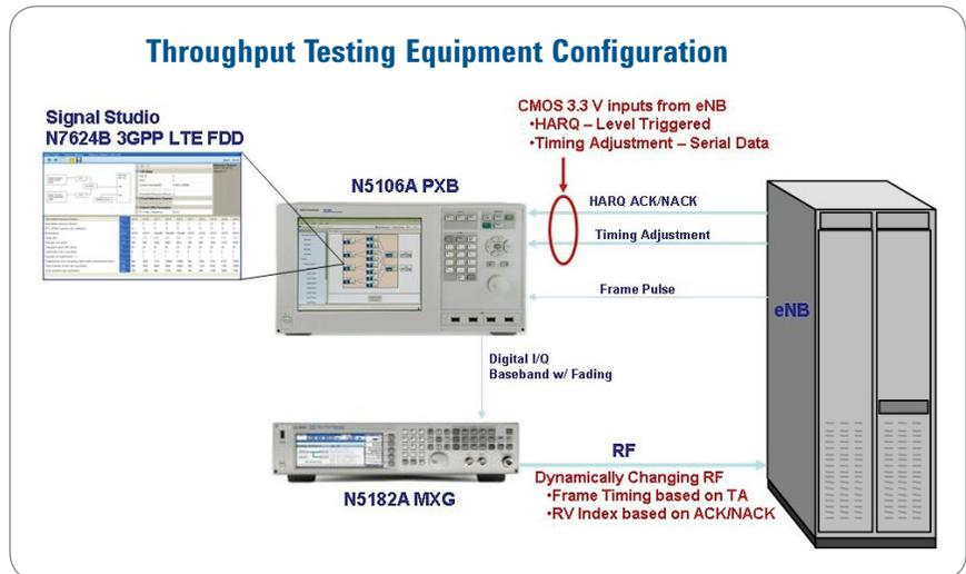
FIGURE 3: The set up shown above of the PXB with MXG and Signal Studio software can be used to perform HARQ and timing adjustment tests in a closed loop manner. Note that while this figure depicts feedback coming over two lines, the signals can be combined into one line, an especially useful ability for eNB hardware that have a limited number of input/output ports available.
