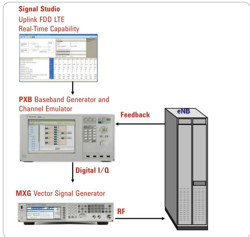
FIGURE 1: The PXB combined with the MXG and Signal Studio software enables efficient LTE eNB conformance testing.
