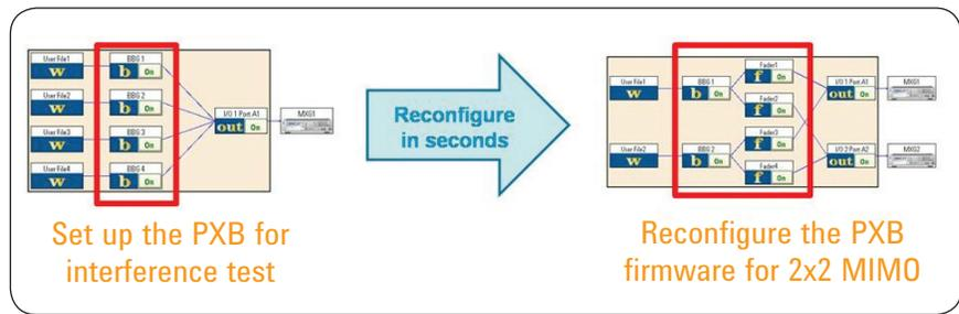
FIGURE 2: The PXB supports over 20 configurations, up to 4x2 MIMO, that can be redefined in seconds.
