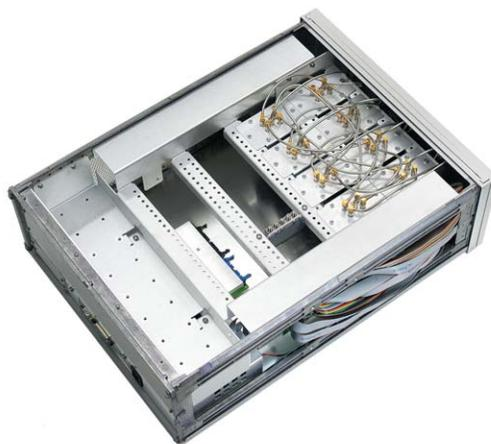
Figure 21. Sample in-house switch matrix design
