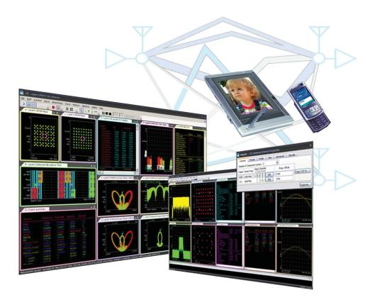
The 89600 VSA software is a window into what is happening inside complex wireless devices. It is equipped to measure more than 70 signal standards and modulation types, including LTE (FDD/TDD), W-CDMA HSPA+, GSM/EDGE Evolution, 802.16 OFDMA and ultra-wideband (UWB) MB-OFDM.
