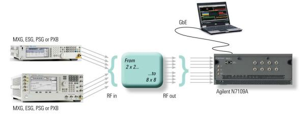
Figure 1. Typical MIMO test setup.
