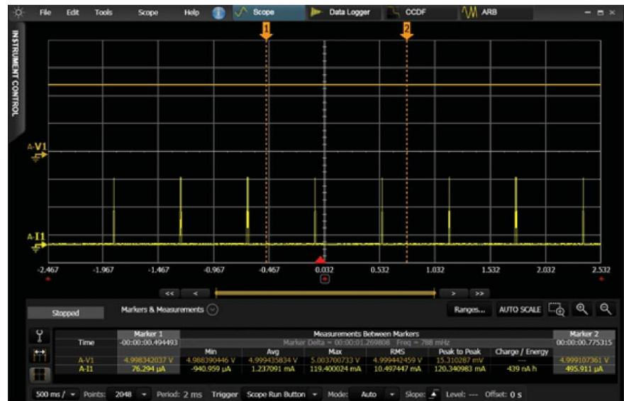
Figure 5: Scope acquisition with markers
