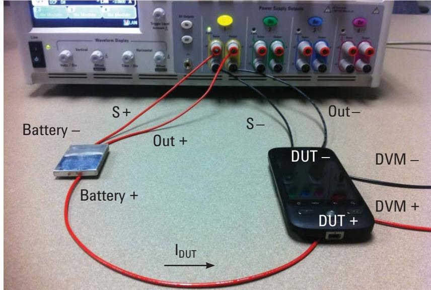
Figure 2: The actual setup for measuring battery run-down performance using the N6781A SMU installed as output 1 in an N6705B DC power analyzer mainframe.
