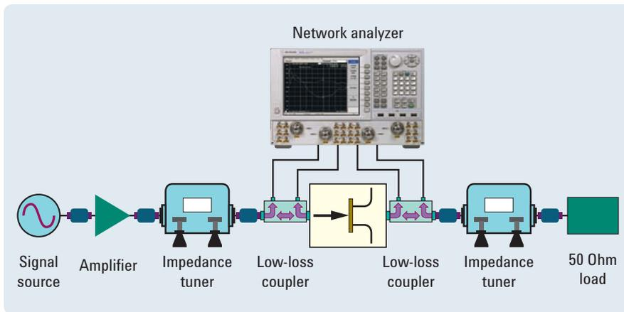
Using a vector-receiver load pull system eliminates the necessity for multiple load-pull source-pull iterations thereby saving time, it reduces errors cause by de-embedding through tuners at higher gammas and it improves the overall accuracy by measuring at the DUT reference plane.
