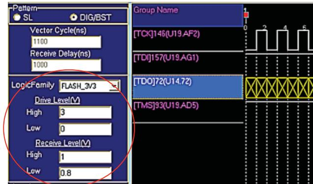
Figure 19. Adjusting logic levels on selected signals
