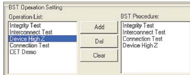
Figure 12. Selecting test types in BST Interface
