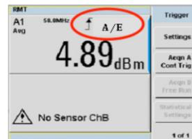
Figure 3. Triggering mode in Internal/External Trigger. (In image, for A/E, A = Internal trigger/E = External trigger)
