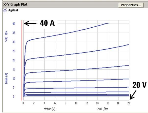
Figure 2. 40A pulsed Id-Vd plot using Id-Vd application test. Note: Two HCSMUs are combined in parallel.
