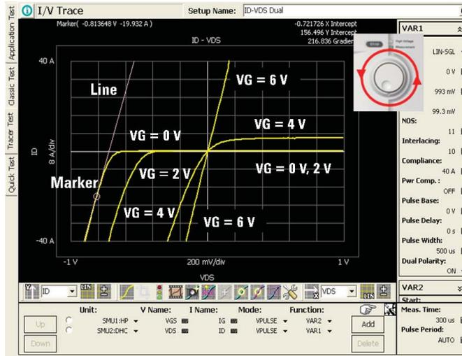
Figure 4. VSD and ISD quadrant sweep using the Tracer Test mode.
