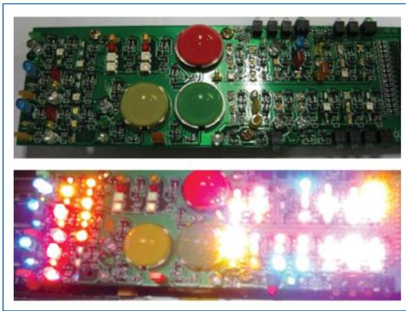
**FIGURE 1.** LED demo board before (top) and after being powered via ICT.
