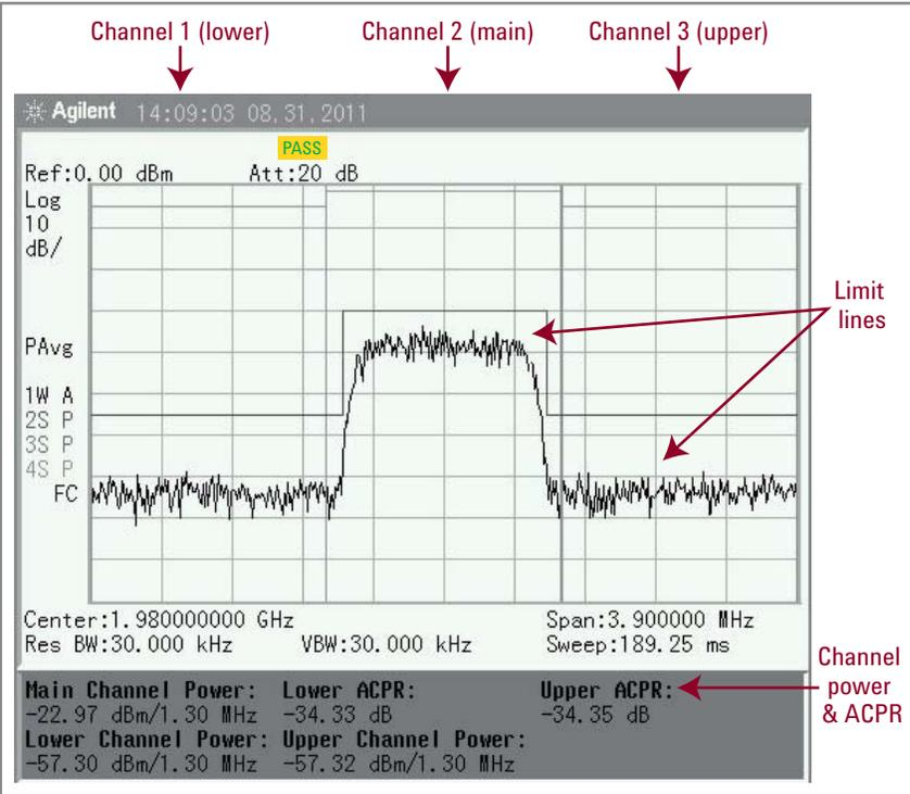
Figure 4. Measurement of adjacent channel power and limit testing
