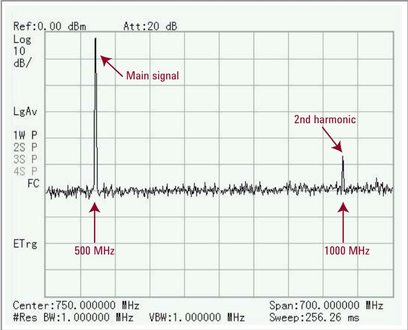
Figure 3. Measurement of 500 MHz unfiltered transmitter showing second harmonic generated at the output
