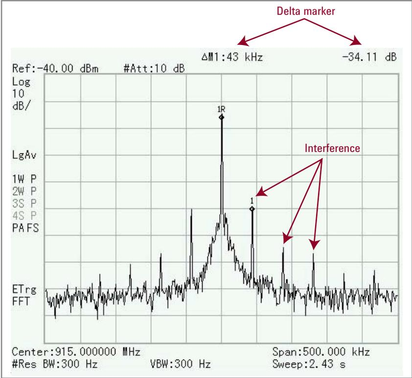
Figure 2. Measured spectrum of a CW carrier showing modulation sidebands creating by fluorescent lighting
