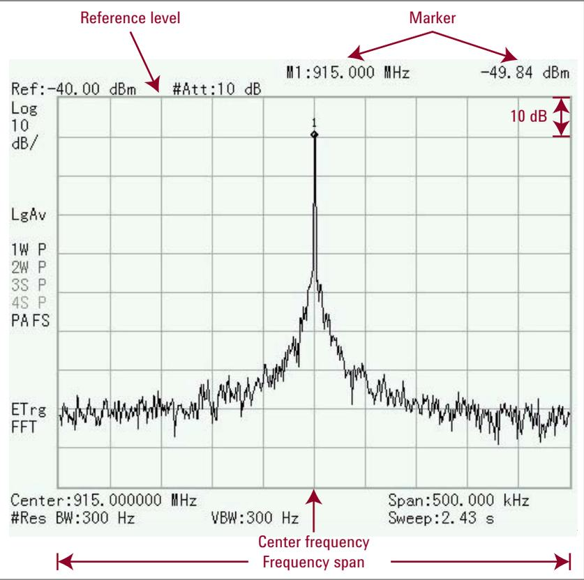
Figure 3. Over-the-air measurement of a 915MHz RF signal in an office environment with the lighting turned off
