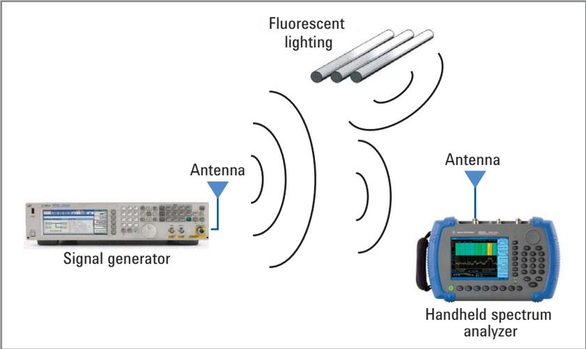
Figure 1. Test configuration for evaluating the affects of fluorescent lighting on a UHF RFID system
