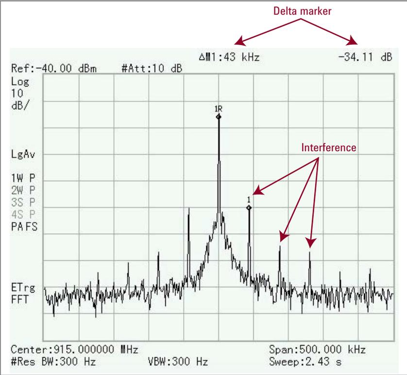
Figure 4. Over-the-air measurement of a 915 MHz RF signal in an office environment with the fluorescent lighting turned on. Shown are the modulation sidebands of the 43 kHz operating frequency of the electronic lighting ballast
