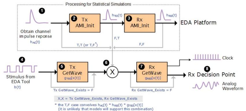
Figure 3. The IBIS-AMI statistical and time-domain reference flow.
