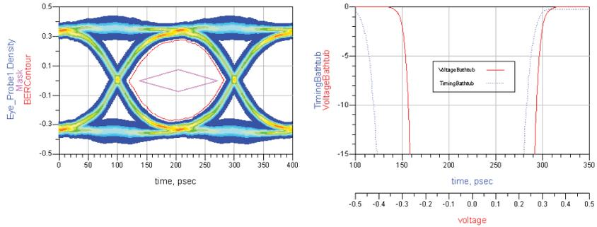
Figure 8. Eye density and bathtub plots with -2.5 dB of Tx equalization.
