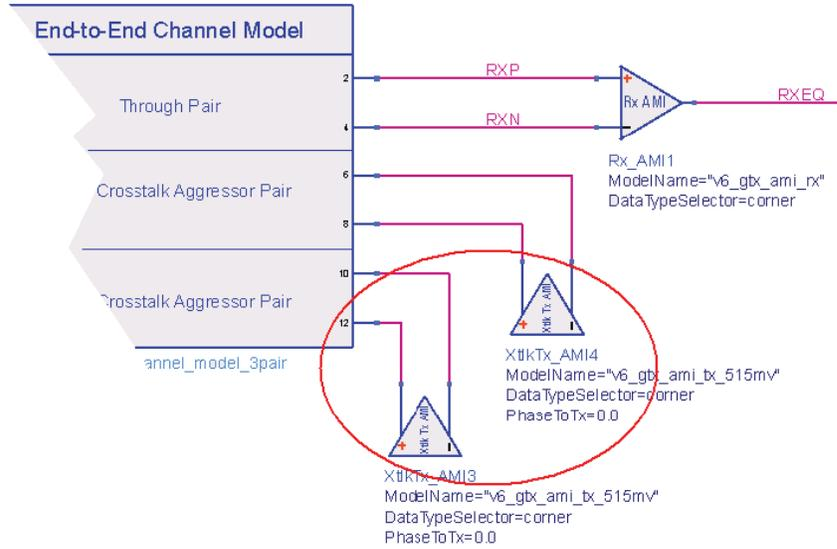
Figure 10. The passive terminations are swapped out with IBIS-AMI NEXT crosstalk transmitters.
