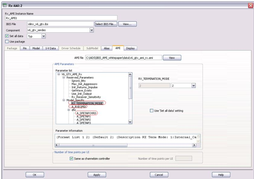
Figure 7. The ADS IBIS-AMI Rx setup dialog.
