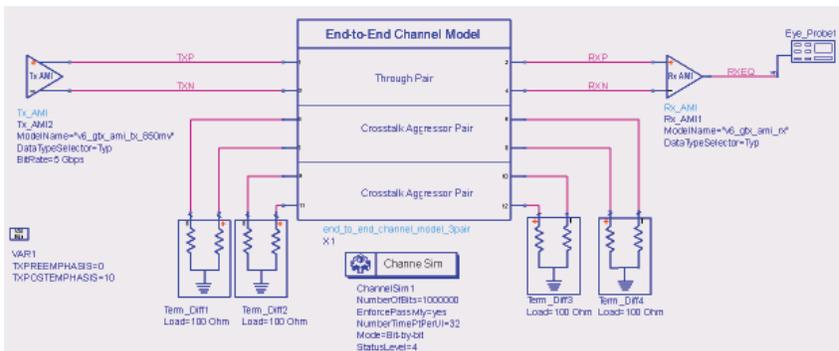
Figure 5. Demonstration channel topology.
