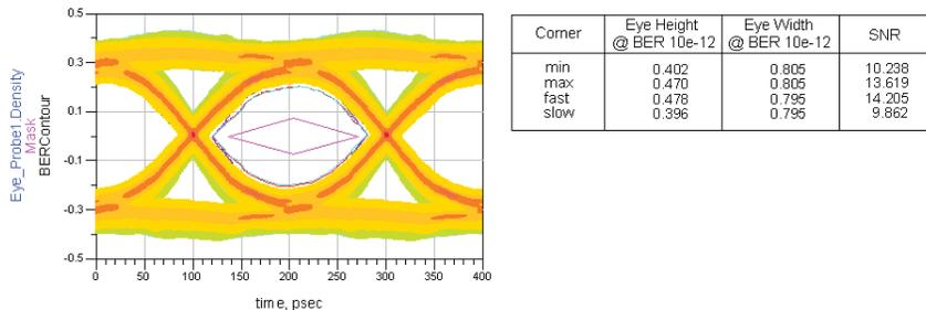
Figure 12. An eye opening over minimum, maximum, fast, and slow corners.
