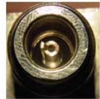
*Figure 10. Damaged female connector fingers*
