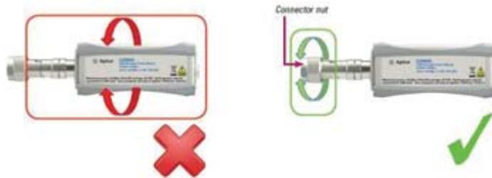
Figure 8. Making connections properly prevents damage to sensors
