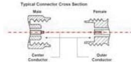
Figure 5. Male and female connector cross section
