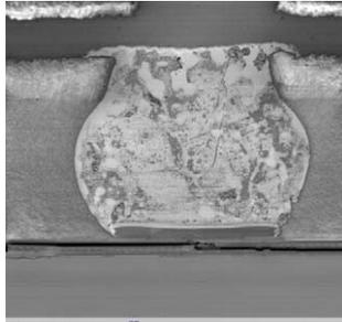
Figure 15. BGA contact pad.
