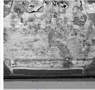
Figure 18. BGA contact pad, IC chip contact interface.
