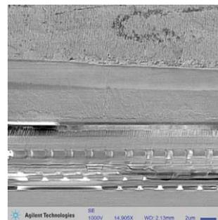
Figure 19. BGA contact pad, IC chip contact interface.
