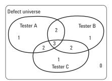
Figure 1. Venn diagram of a defect universe and how 3 different test technologies may cover it. The number of testers that may test a given defect are shown.
