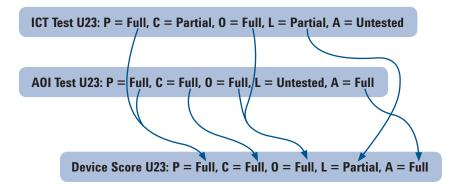
Figure 4. Device property coverage scored by two tests of differing capabilities.
