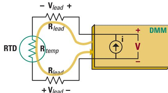
Figure 4: A two-wire RTD measurement
