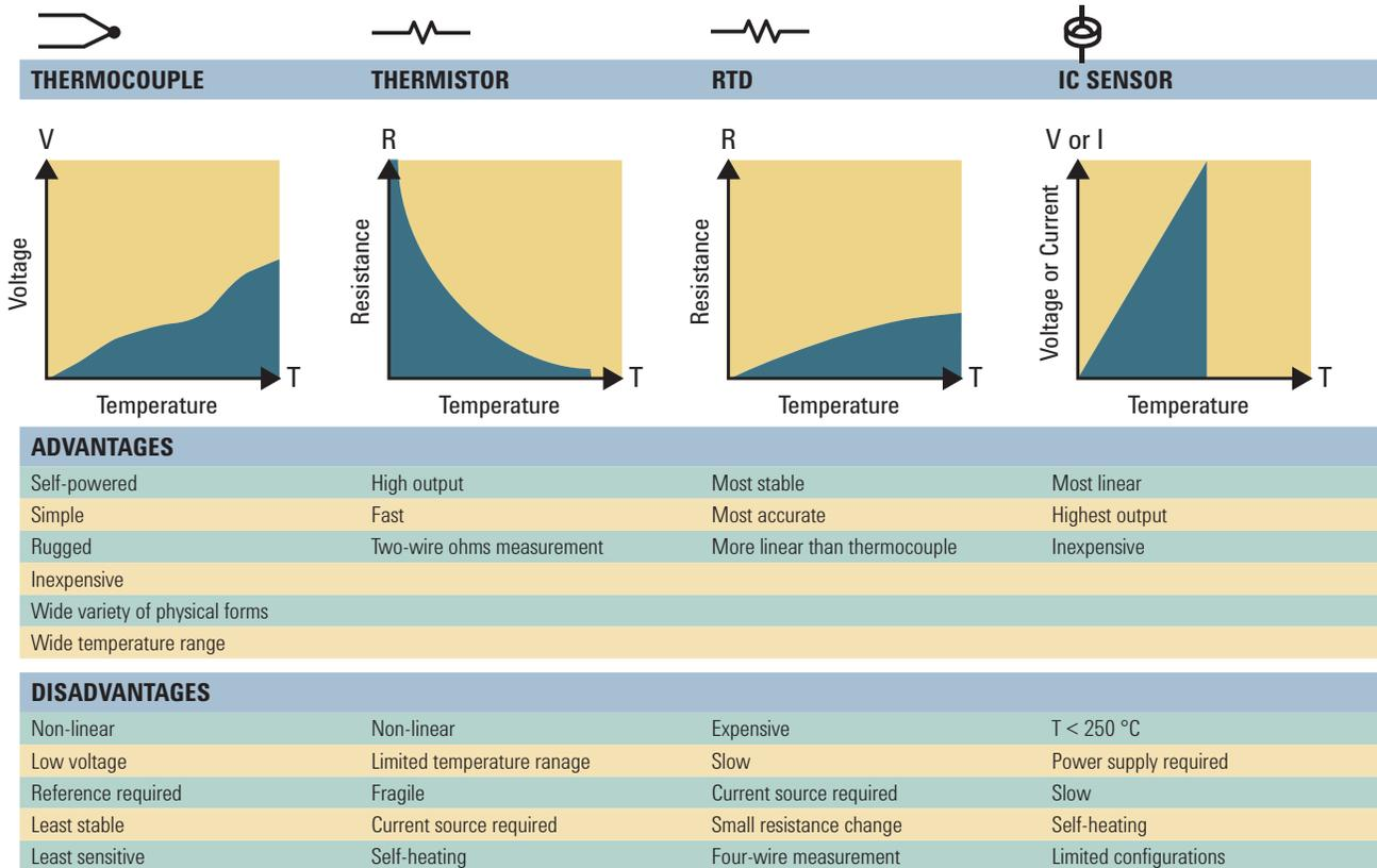
Figure 1: Advantages and disadvantages of popular temperature sensors
