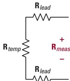
Figure 3: Thermistor schematic
