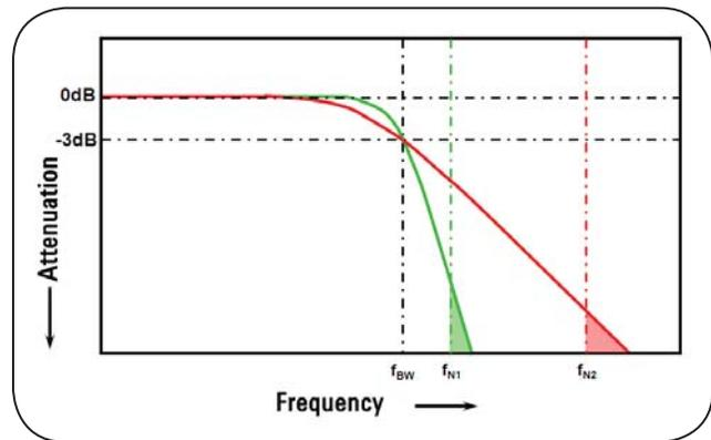
Figure 8: Typical oscilloscope frequency responses.
