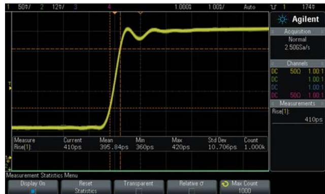
**Figure 4: Capturing a fast rising edge at 2.5 GSa/s with automatic  $\sin(x)/x$  waveform reconstruction.**
