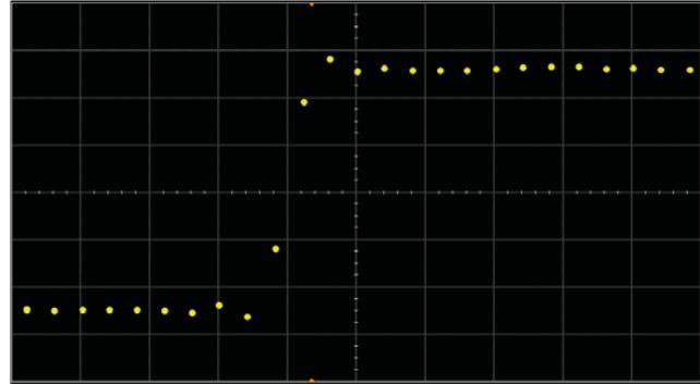
**Figure 3: Single-shot capture of a fast rising edge sampled at 2.5 GSa/s, but without digital waveform reconstruction filtering.**
