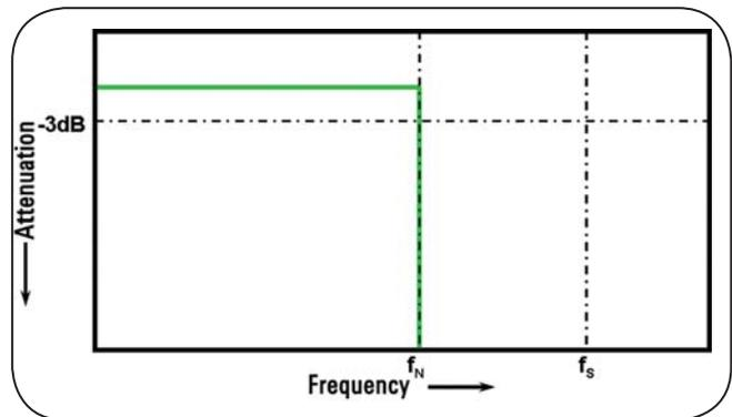
Figure 7: Theoretical brick-wall frequency response.
