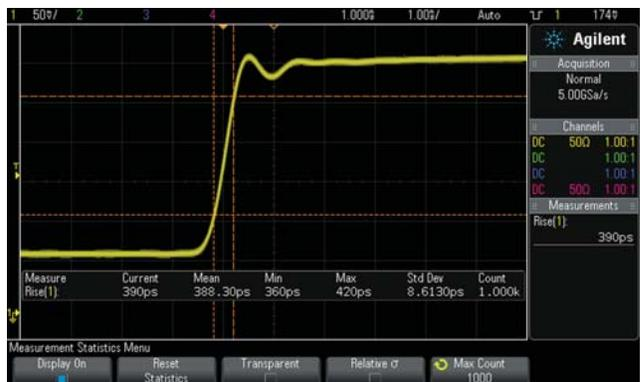
**Figure 5: Capturing a fast rising edge at 5 GSa/s with automatic  $\sin(x)/x$  waveform reconstruction.**
