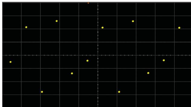
**Figure 1: Single-shot capture of a 1-GHz sine wave sampled at 2.5 GSa/s, but without digital waveform reconstruction filtering.**
