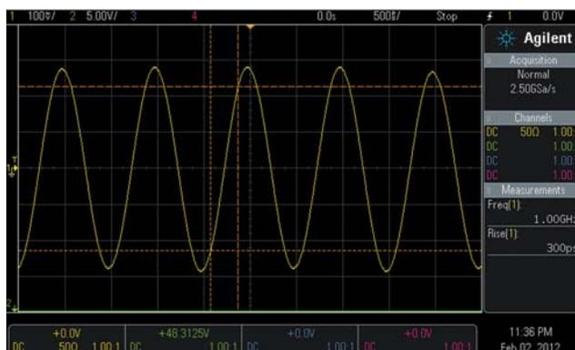
**Figure 2: Single-shot capture of a 1-GHz sine wave at 2.5 GSa/s with sin(x)/x reconstructed samples.**
