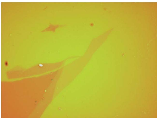
Figure 1. An optical photograph of exfoliated graphene flakes with various thickness on a silicon dioxide substrate.
