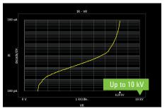
The Ultra High Voltage Unit can accurately measure both breakdown voltage at up to 10 kV and small leakage current at up to 10 kV with pA resolution.
