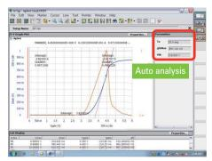
Powerful auto-analysis capability permits the easy and accurate extraction of device parameters such as power MOSFET transconductance (Gm) and threshold voltage.
