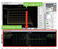
The High Voltage Medium Current Unit can make Id-Vd curves (such as 500 mA at 1200 V) with unparalleled accuracy. The Oscilloscope view feature allows you to verify your measurement pulses and timings without an oscilloscope.
