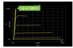
Ic-Vc characteristics of IGBT modules can be measured accurately at collector current levels up to 1500 A using the Ultra High Current Unit.
