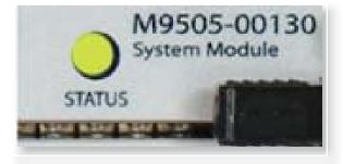
Figure 2. AXIe status light on ESM module must be green before powering-up controller.
