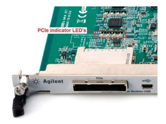
Figure 5. AXIe chassis: LED's on M9505A ESM indicate PCIe bus connectivity.
