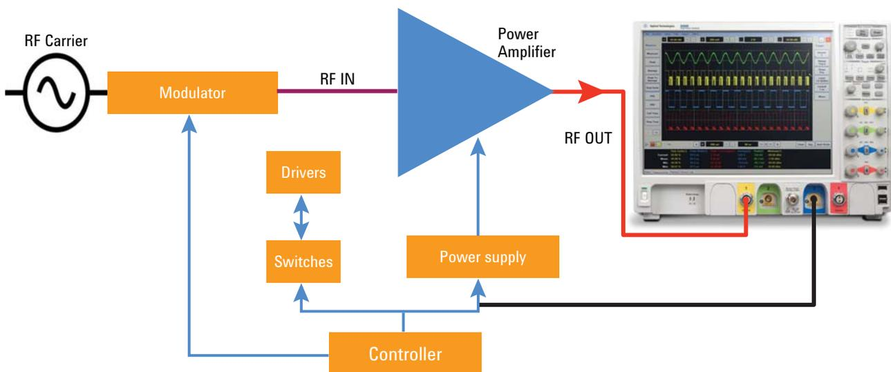
Figure 7. Analyzing timing information of RF burst and control signals
