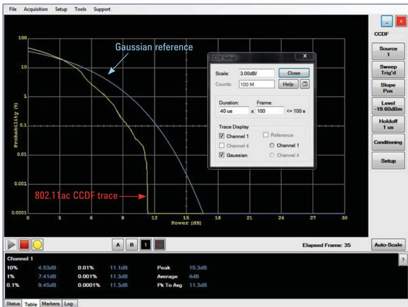
Figure 5. 802.11ac CCDF plot obtained using an 8990B PPA
