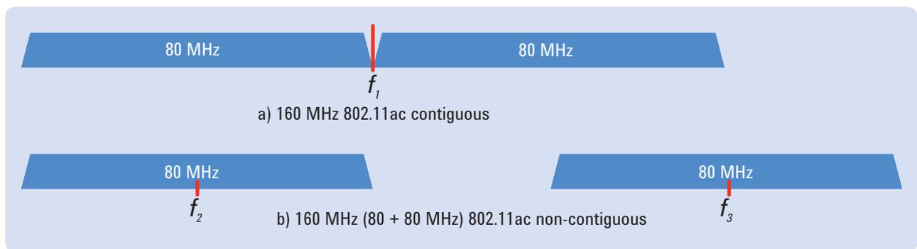
Figure 1. 802.11ac 160 MHz bandwidth channelization
