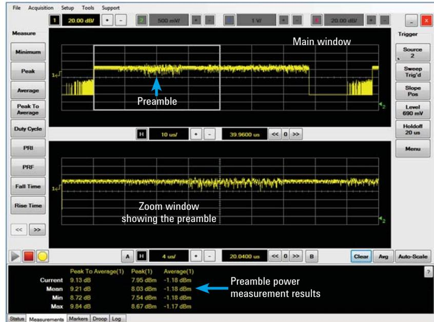
Figure 3. 802.11ac 80MHz bandwidth preamble power measurement
