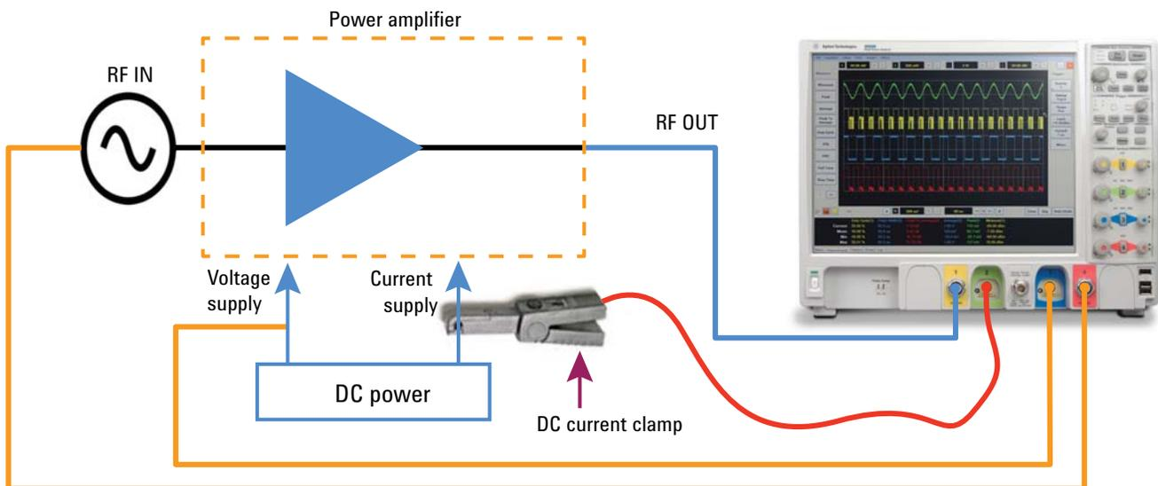
Figure 6. Power added efficiency test setup
