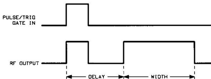
This modulation source requires an external trigger source.
