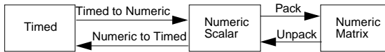
Figure 5-3. Timed Data Must be Converted to Numeric Scalar Before Being Converted to Matrix
